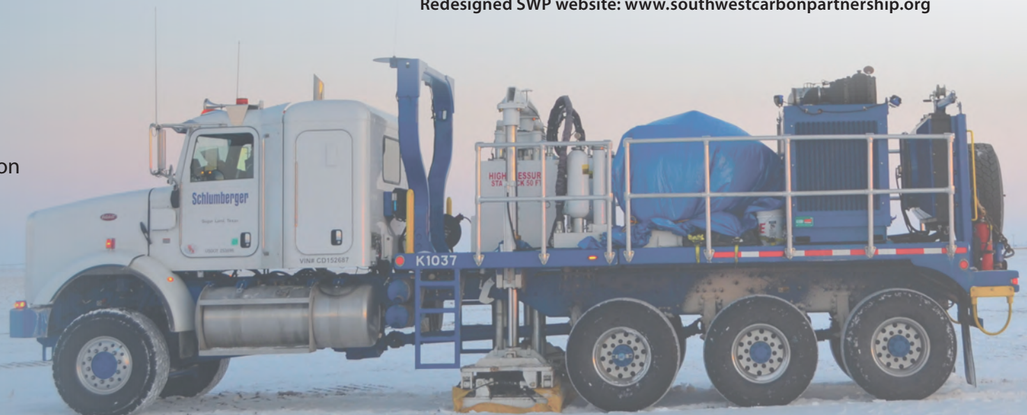
Background image: VSP survey being conducted by Schlumberger Q-Borehole Explorer vibrator truck at the Farnsworth Unit.
